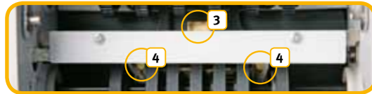
3 Infrared / UV-sensor 4 Right and left counter sensor
